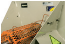
External lubricators to facilitate maintenance
